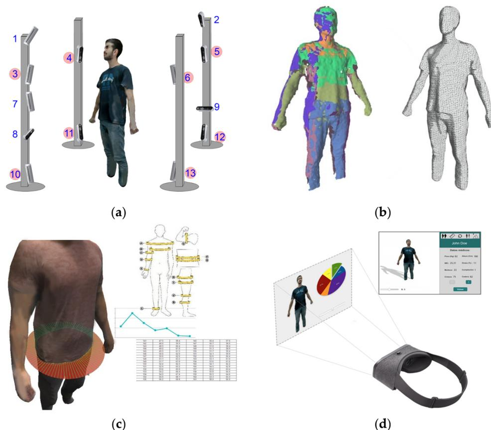
**Figure 1.** Proposed framework system based on an RGB-D camera network (a). Body models: point clouds and mesh (b). 3D body measurement (c) and textured representation with virtual reality (VR) devices (d).
