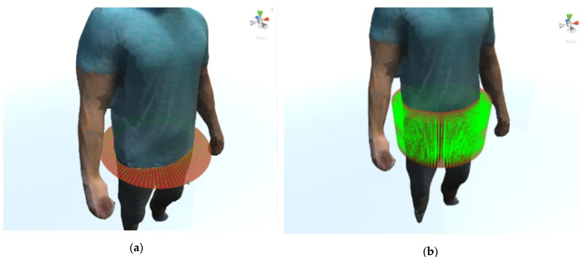
**Figure 9.** Rays perpendicularly launched along the circumferential chord of the circle storing the points of collision with the mesh (a). Rays perpendicularly launched along the circumferential chord of the circles inside the cylinder storing the points of collision with the mesh (b).
