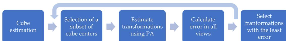
Figure 3. Pipeline of the calibration method based on 3D markers.
