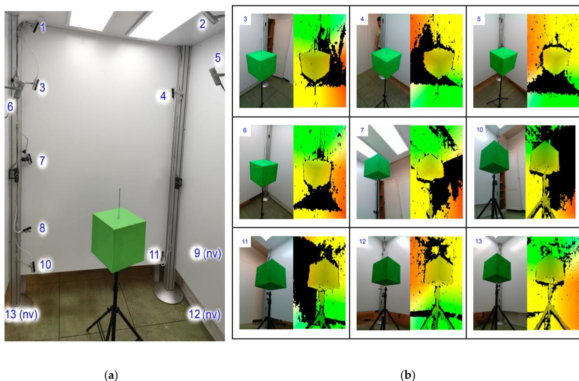
**Figure 2.** (a) Experimental set-up 13 RGB-D cameras. “nv” means a camera not visible in this image. (b) Acquisition results for the cameras (color and depth images). The green cube has been used for extrinsic calibration. Images from high, intermediate and super-low levels are shown.
