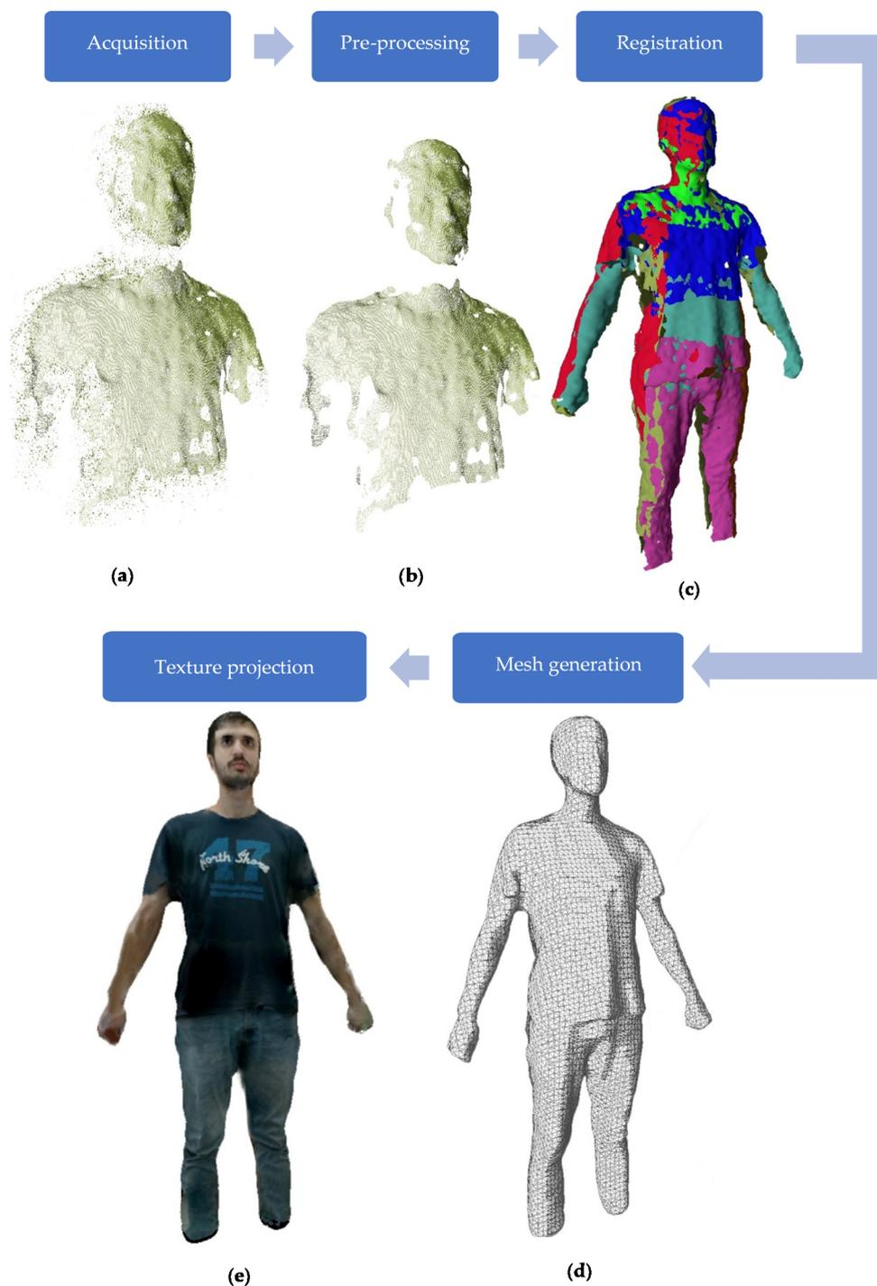
**Figure 4.** Pipeline of 3D body reconstruction. The system is able to acquire several images from cameras (a) that are preprocessed in order to improve the quality of the acquisition (b). The set of points are registered in a single coordinate system (c). Finally, in order to obtain the dense 3D model of the body, the 3D points are converted into a mesh (e) and the color images that were captured synchronously with the point cloud are texture-mapped onto the mesh (d).
