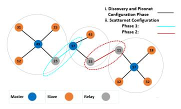
Figure 3. Cluster-based On Demand Routing Protocol [10].
