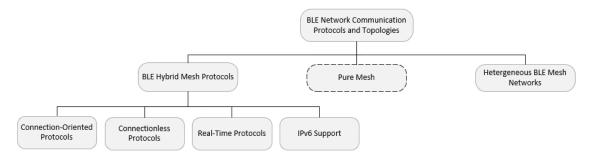
Figure 2. Classification of BLE Communication Protocols.
