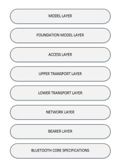
Figure 1. Bluetooth Low Energy (BLE) Mesh System Architecture [17].
