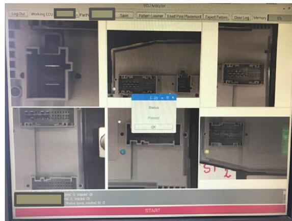
**Figure 23.** An overview of the user interface and a test result for no detected faults.
