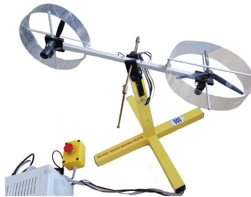
Figure 1. A nonlinear twin-rotor MIMO system.
