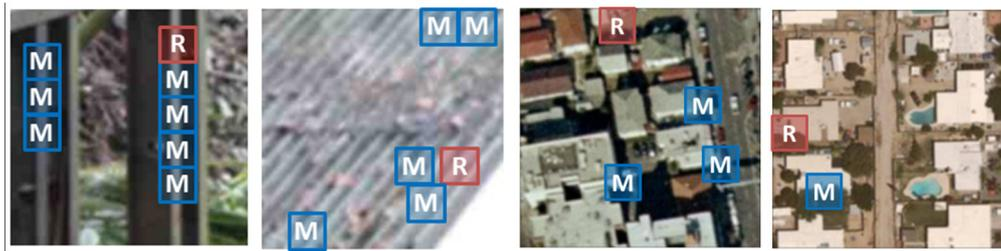
**Figure 3.** Illustration of grouping blocks from degraded natural images/RS scene images corrupted jointly by Gaussian blur and JPEG compression. Each fragment shows a reference block marked with “R” and a few of the blocks matched to it with “M.”.
