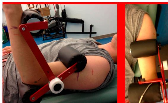
Figure 4. Testing set-up of LSMD in flexion (left) and extension (right).
