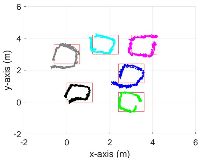
Figure 9. Node tracking performance of the eCDRO-SLAM for Experiment 1.
