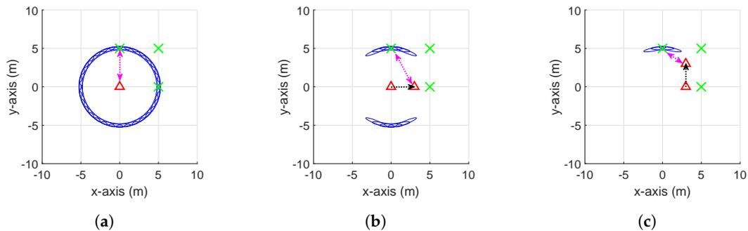
**Figure 1.** Explanation of the conventional RO-SLAM algorithms. Red triangles and green crosses indicate robots and neighbor nodes, respectively. Black and magenta dotted lines are the movement of the robot and range measurements, respectively. Blue ellipse is a possible location of nodes. The conventional RO-SLAM algorithms involve (a) the initial localization when receiving the first measurement, (b) movement of a robot to disambiguate the x-axis, and (c) movement to disambiguate the y-axis.
