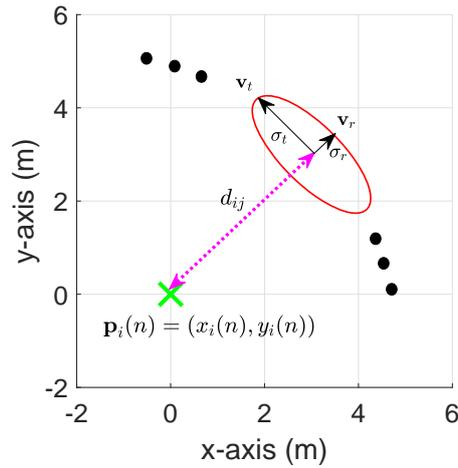
**Figure 4.** Generation of SoG variables. The dotted magentaline represents the measurement.  $\mathbf{v}_r$  and  $\mathbf{v}_t$  are, respectively, the radial and tangential unit vectors, and  $\sigma_r$  and  $\sigma_t$  denote, respectively, the radial and tangential standard deviations.
