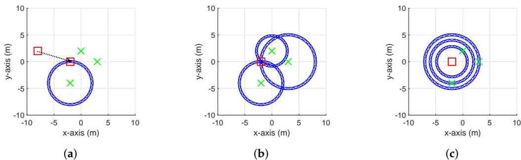
**Figure 2.** Description of the updated procedures for tracking moving nodes. (a) Reset the SoG variables from the neighbor node to the moving node, (b) update and merge the SoG variables, and (c) reset the SoG variables from the moving node to its neighbor nodes and update the corresponding weights. The red squares and green crosses represent the moving nodes and neighbor nodes, respectively. The black dotted line represents the movement of a node.
