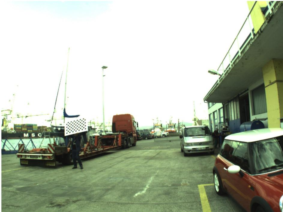
**Figure 3.** Calibration of a stereo system that is mounted on an unmanned surface vehicle (USV) is a completely different endeavour than calibrating the stereo rig in the laboratory. Note that “in the wild” it is practically impossible to cover the whole image area with the calibration target, unless one of the operators is able to climb while holding the target.
