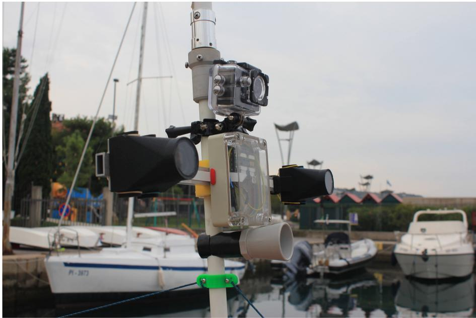
**Figure 2.** Our stereo system mounted on the USV.
