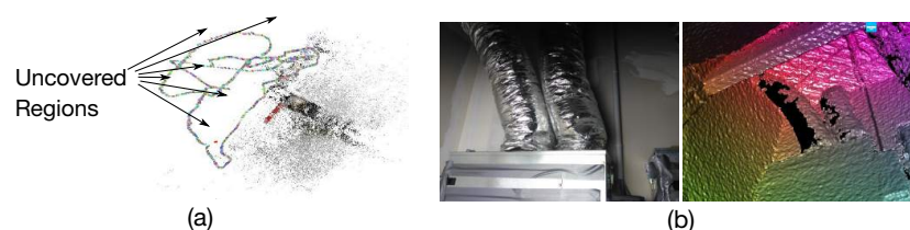
Figure 1. Challenges of collecting training data in industrial environments. (a) There are some uncovered regions within the training data using traditional video collection [6]. (b) There are some missing parts within the reconstructed 3D model on specular surfaces using Kinect Fusion [23,24].
