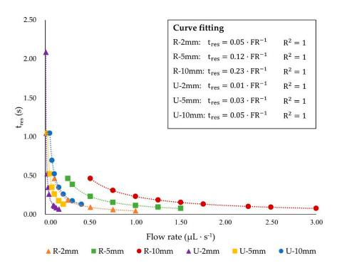
Figure S2. Variation of the residence time with the fluid flow rate for all of the studied geometries.
