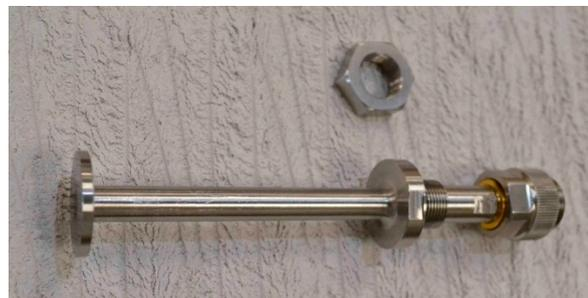
**Figure 3.** Photograph of one of the 7-mm open-ended coaxial probes. Probe A is shown, but Probe B is of identical design.
