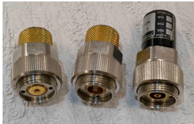
**Figure 4.** GPC-7 impedance standards (left to right: short-circuit, open-circuit and low-band load).
