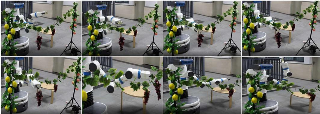
**Figure 13.** Video frames showing the robot reaching a cluster of plastic grapes, cutting the peduncle, and placing them onto a table.
