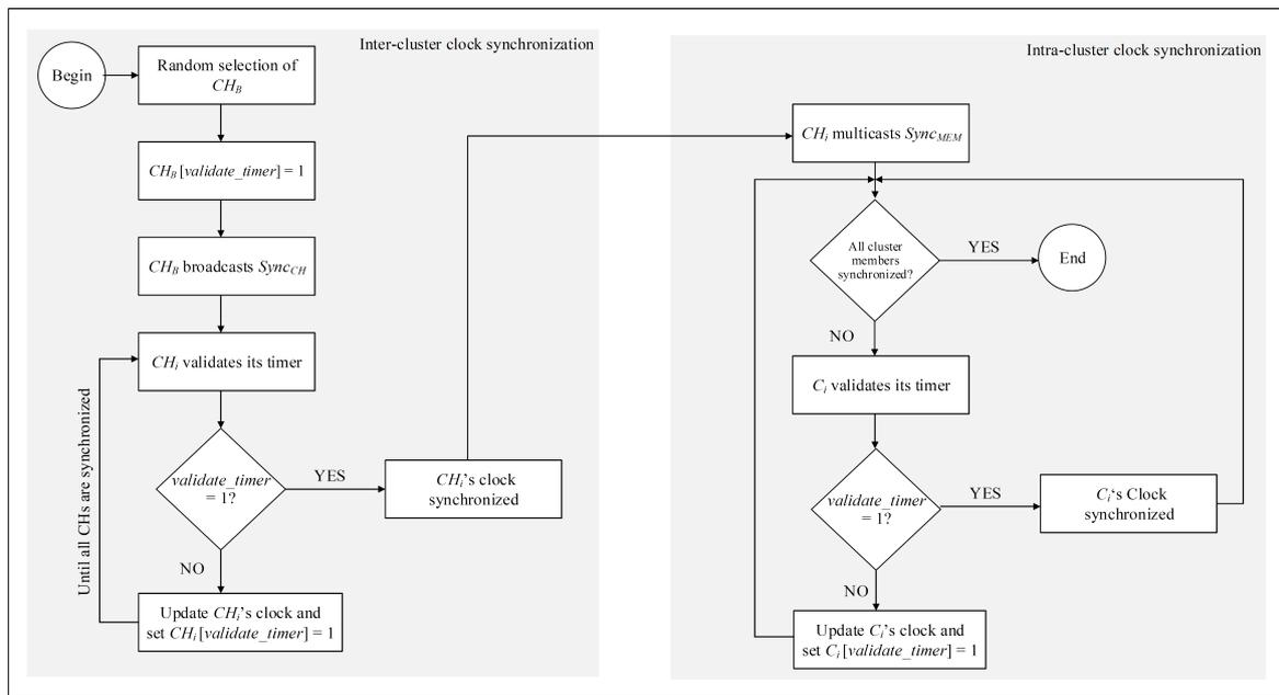
**Figure 3.** Procedural flowchart of the clock synchronization algorithm.
