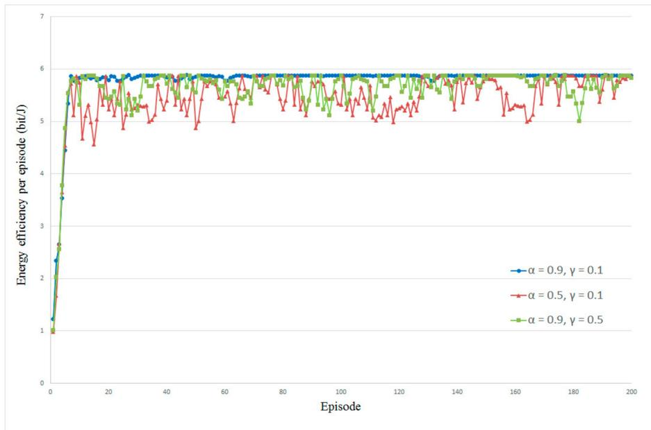
**Figure 2.** Influence of  $\alpha$  and  $\gamma$  on energy efficiency in direct transmission mode.
