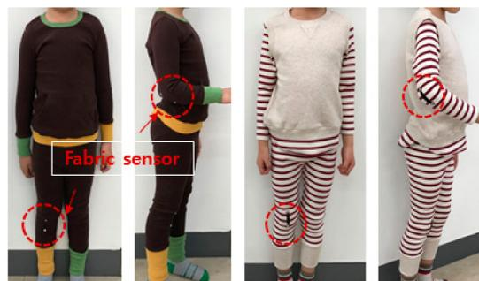
**Figure 5.** Examples of developed test clothing with integrated fabric motion sensor.
