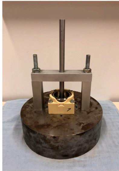
**Figure 2.** Guiding system to insert the implant in the acetabular models.
