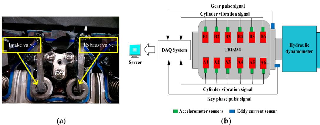
**Figure 6.** Valve train and the main test rig components: (a) intake valve and exhaust valve and (b) the sketch of diesel engine test rig and sensors positioning.
