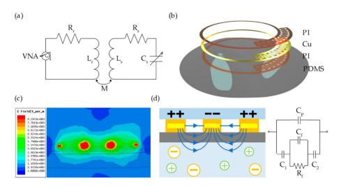
**Figure 1.** (a) Illustrative model schematic of resistor–inductor–capacitor (RLC) wireless measurement; (b) structural schematic of the proposed dielectric sensor; (c) electric field leaked out between the interdigital electrodes on high-frequency structure simulator (HFSS) simulation; and (d) schematic and equivalent circuit of the fluid monitoring.
