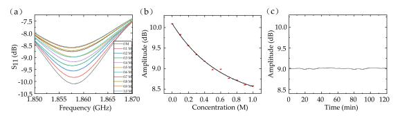
**Figure 6.** The  $S_{11}$  (**a**) and fitting results (**b**) of the NaCl solutions with different concentrations. (**c**) The sensor's stability with 0.5 M NaCl solution injected.
