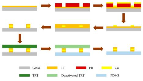
Figure 2. Fabrication process of the proposed RLC dielectric sensor.
