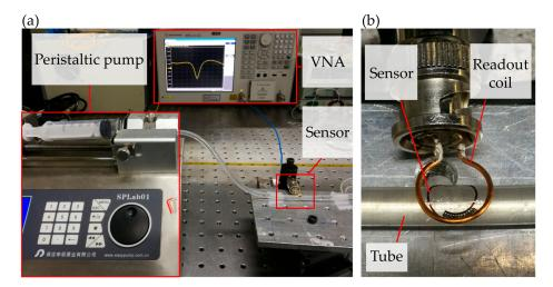
**Figure 4.** Experimental setup of the dielectric sensor monitoring the fluid. (**a**) Picture of the testing platform for the dielectric sensor. (**b**) Picture of the sensor stuck on the tube and communicated with the readout coil.
