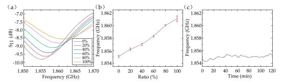
**Figure 5.** The  $S_{11}$  (**a**) and fitting results (**b**) of the ethanol/water solutions with different ethanol's volume fraction. (**c**) Sensor's stability with pure water injected.
