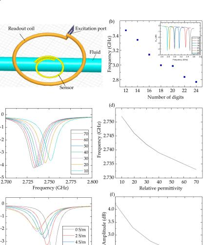
Figure 3. HFSS simulation of the dielectric sensor monitoring the fluid. (a) Model of the HFSS simulation and (b) the sensor's resonant frequency with 12-24 digits. The  $S_{11}$  (c) and fitting results (d) of the fluid with different relative permittivities. The  $S_{11}$  (e) and fitting results (f) of the fluid with different conductivities.
