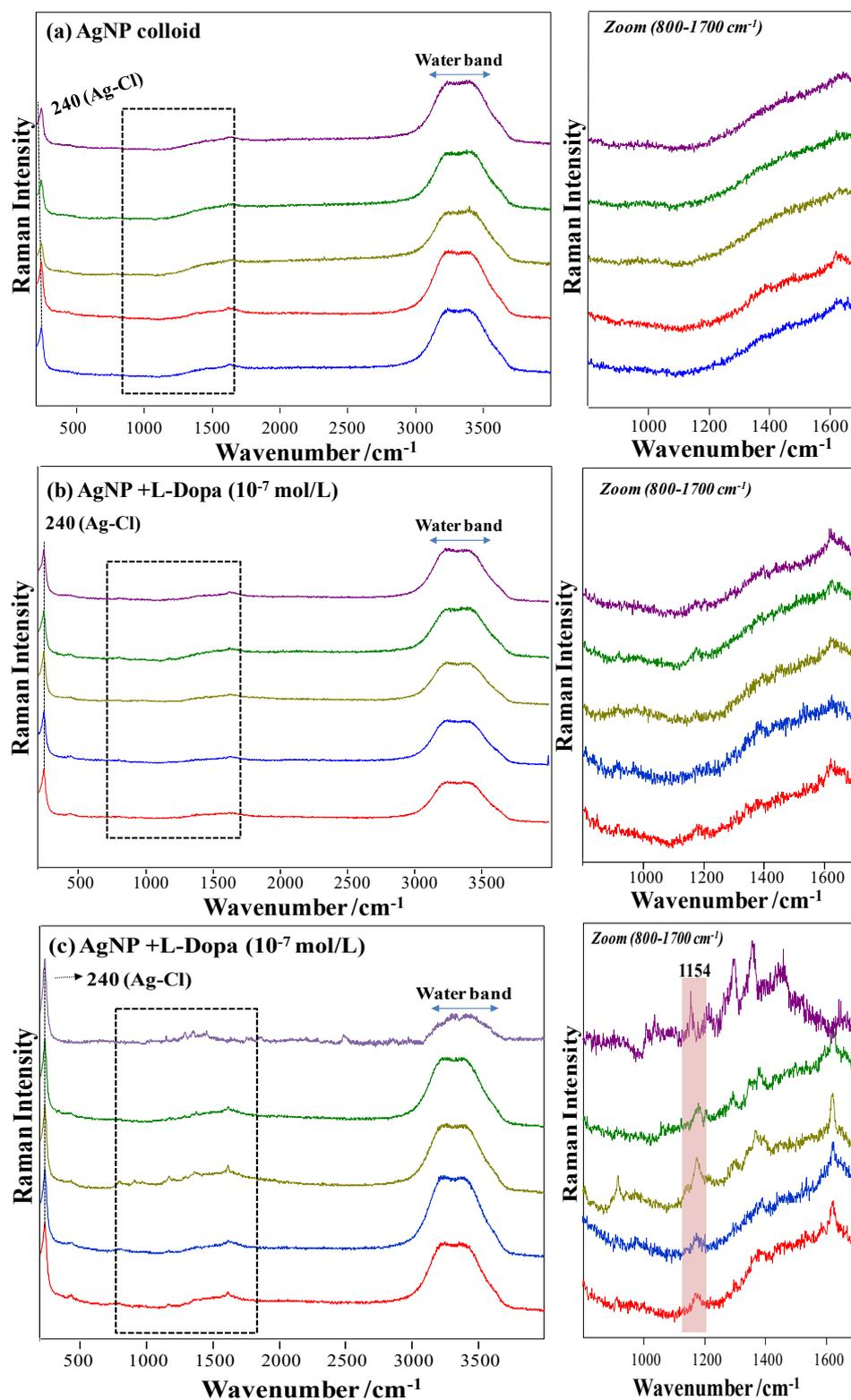
**Figure S1.** (a) Raman spectra of AgNP colloidal suspensions. (b) SERS spectra of AgNP colloidal suspensions in the presence of  $10^{-7}$  mol/L of L-Dopa showing no active L-Dopa SERS signal. (c) SERS spectra of AgNP colloidal suspensions in the presence of  $10^{-7}$  mol/L of L-Dopa showing the L-Dopa SERS signal, which corresponds to ca. 5% of all spectra recorded. The highlighted band at 1154  $\text{cm}^{-1}$  (Figure S1c) was used to calculate SNR (SNR = 3.3). Laser line at 633 nm.
