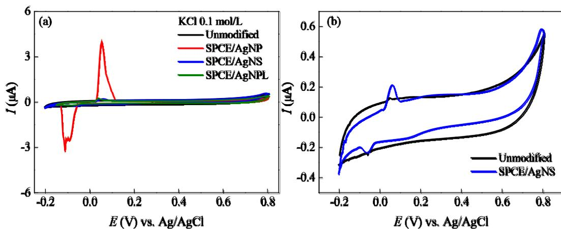
**Figure S6.** (a) Cyclic voltammetry of SPCE unmodified and modified with AgNP, AgNS and AgNPL in 0.1 mol/L KCl solution. (b) Cyclic voltammetry of SPCE unmodified and modified with AgNS from Figure S6 (a) for better view.  $v = 25$  mV/s.
