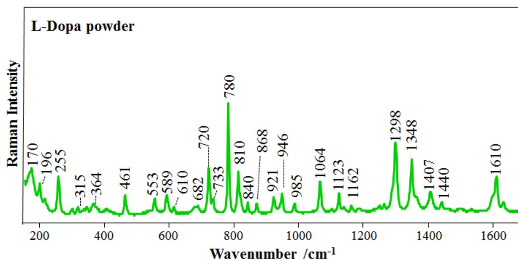
Figure S3. Raman spectrum of L-Dopa powder. Laser line at 633 nm.
