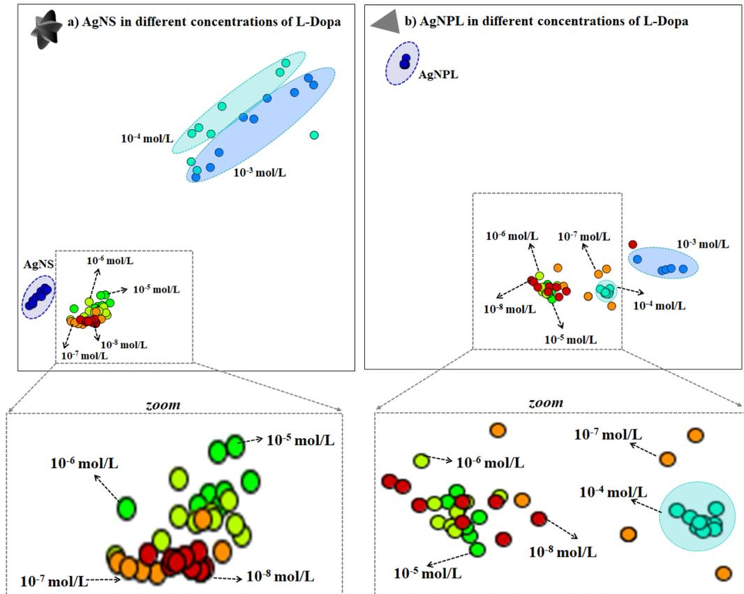
**Figure S5.** Zoom of the IDMAP multidimensional projection for concentrations of L-Dopa (a) down to  $10^{-5}$  mol/L in colloidal suspension of AgNS and (b) down to  $10^{-4}$  mol/L in colloidal suspension of AgNPL. Each circle in the plot represents a whole SERS spectrum. The proximity of the circles indicates the similarity between the SERS spectra.
