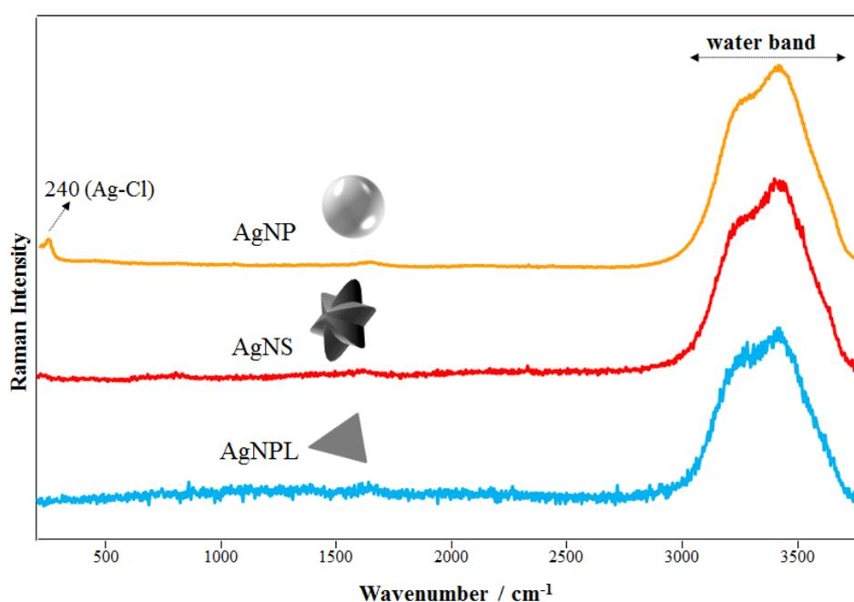
**Figure S2.** Raman spectra of AgNPs, AgNS and AgNPL colloidal suspensions (as reference).
