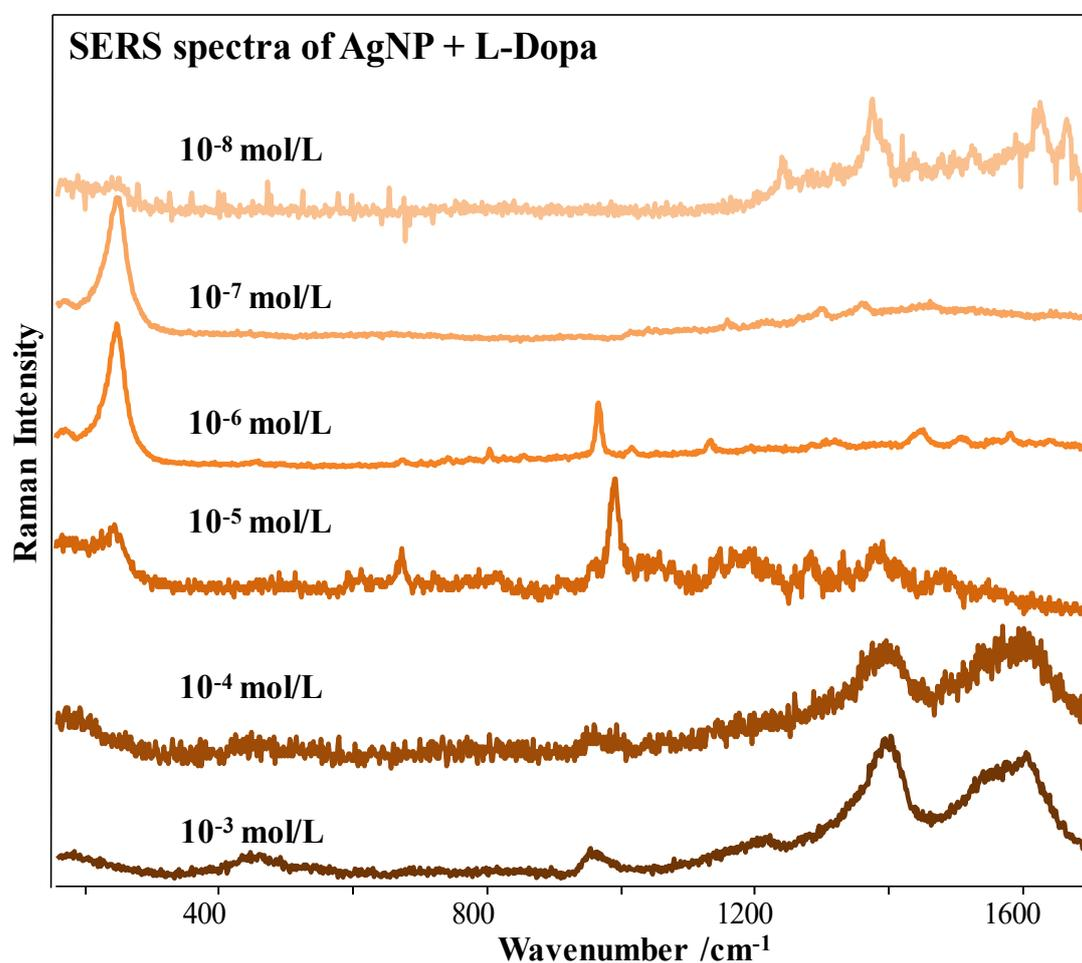
**Figure S4.** SERS spectra of L-Dopa solutions in colloidal suspension of AgNP at different concentrations (from  $10^{-3}$  to  $10^{-8}$  mol/L). Laser line at 633 nm.
