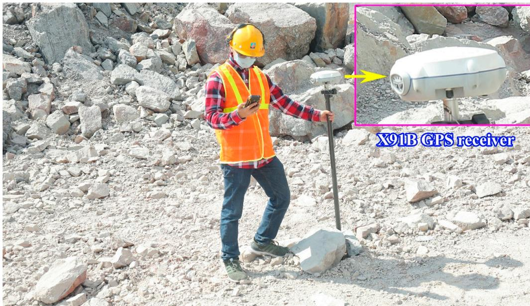
Figure 7. X91B GPS receiver used for measuring the distance in this study.
