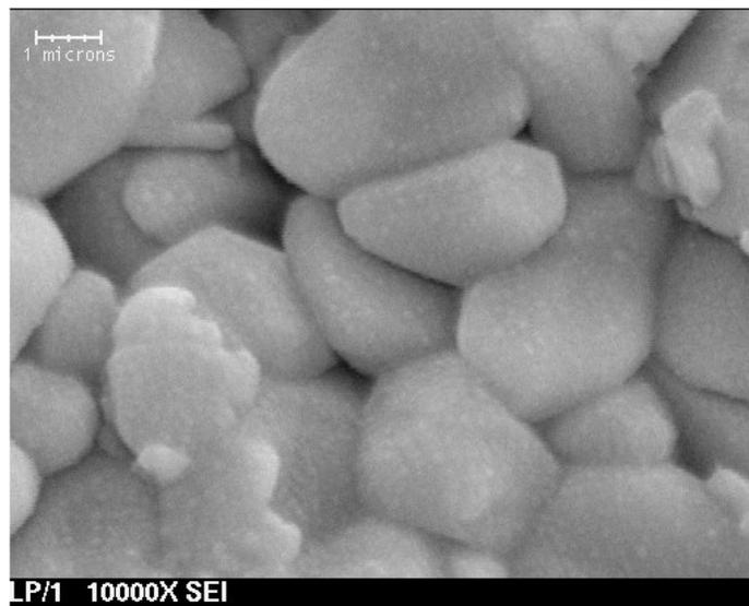
**Figure 2.** SEM Image of the surface of the In<sub>2</sub>O<sub>3</sub>/SiO thin films obtained at a magnification of 10,000.
