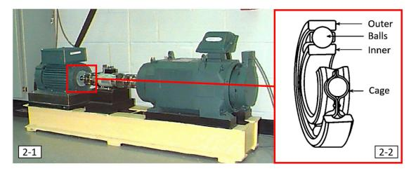
Figure 2. The introduction of experimental platform for the ball-bearing system.
