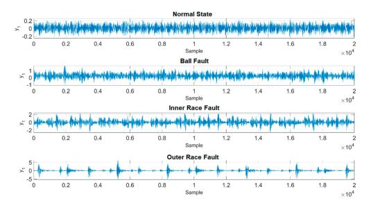
Figure 5. Time series of original vibration data (y).
