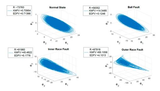
**Figure 10.** The experimental results for the training stage—3D phase portraits. KMFV, K-means-based feature value; EDFV, Euclidean distance feature value.
