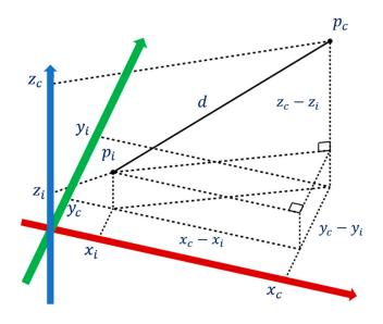
Figure 9. The schematic diagram of 3D Euclidean Distance.
