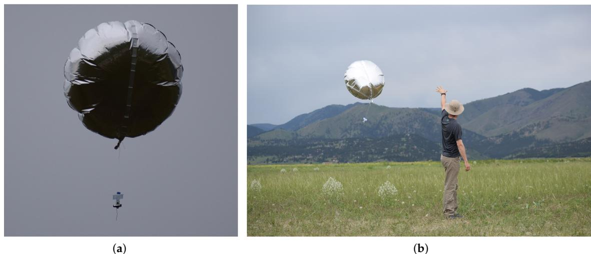
**Figure 1.** Pseudo-Lagrangian drifters (PLD). (a) PLD with attached microsonde. (b) Ground release of a PLD near Boulder, CO, USA. Photo credit: Roger Laurence, University of Colorado.
