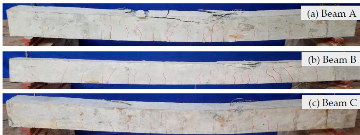
Figure 7. Failure photos of the test specimens.
