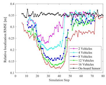
Figure 11. Effect of the number of connected vehicles on perception accuracy.
