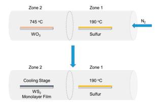
Figure S3. Simplified schematic depicting WS2 fabrication.
