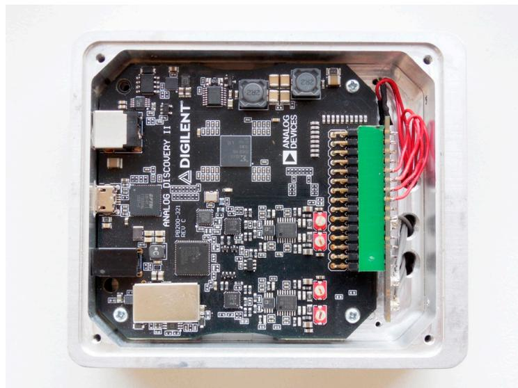
**Figure A3.** A photograph of the signal processing module with Analog Discovery 2 (bottom cover of the analyzer is removed).
