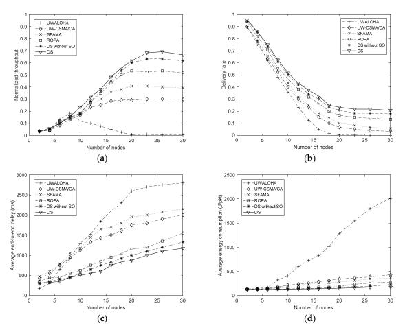
**Figure 4.** Performance of UWALOHA, UW-CSMA/CA, SFAMA, and ROPA protocols and that of the proposed method under different network sizes. (a) Normalized throughput; (b) Packet delivery rate; (c) Average end-to-end delay; (d) Average energy consumption.
