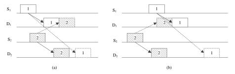
Figure 2. Concurrent transmissions with different sending sequences. (a)  $S_1$  sends first; (b)  $S_2$  sends first.
