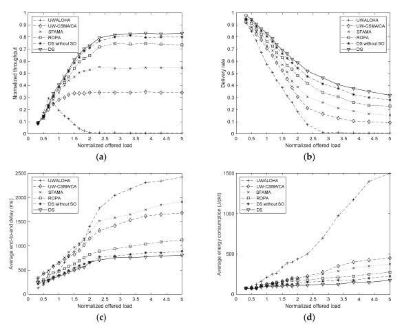
**Figure 3.** Performance of UWALOHA, UW-CSMA/CA, SFAMA, and ROPA protocols and that of the proposed method under different network loads. (**a**) Normalized throughput; (**b**) Packet delivery rate; (**c**) Average end-to-end delay; (**d**) Average energy consumption.
