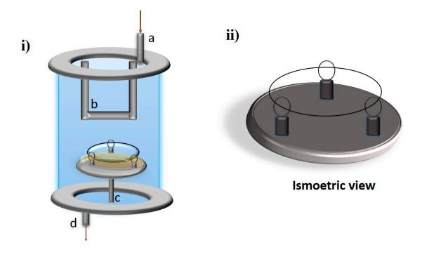
**Figure S1.** i) Schematic of plasma reactor with an additional holder for suspending fiber a) monomer inlet b) RF cathode c) RF anode with attached holder d) monomer outlet ii) Schematic of custom-built fiber holder (isometric view).
