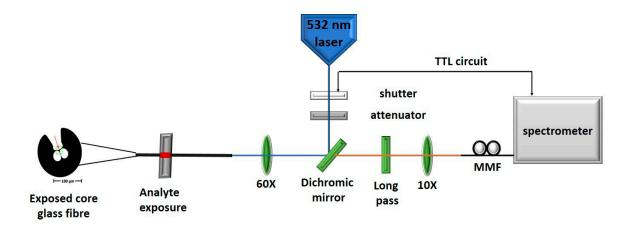
**Figure S3.** Schematic of the optical setup used to measure fluorescence from functionalized exposed core fiber (ECF) when exposed with the Al<sup>3+</sup> ions. A 532 nm laser was used for alignment and for all measurements. The fibers were exposed to Al<sup>3+</sup> ions by immersing a part of the fiber, as is demonstrated in the above figure.
