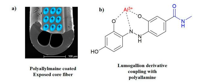
**Figure S2.** a) Schematic showing exposed core fiber (ECF) coated with plasma polymerized allylamine. b) Simplified version of lumogallion derivative coupling with plasma polymerized ECF. (Adapted from Reference 14)
