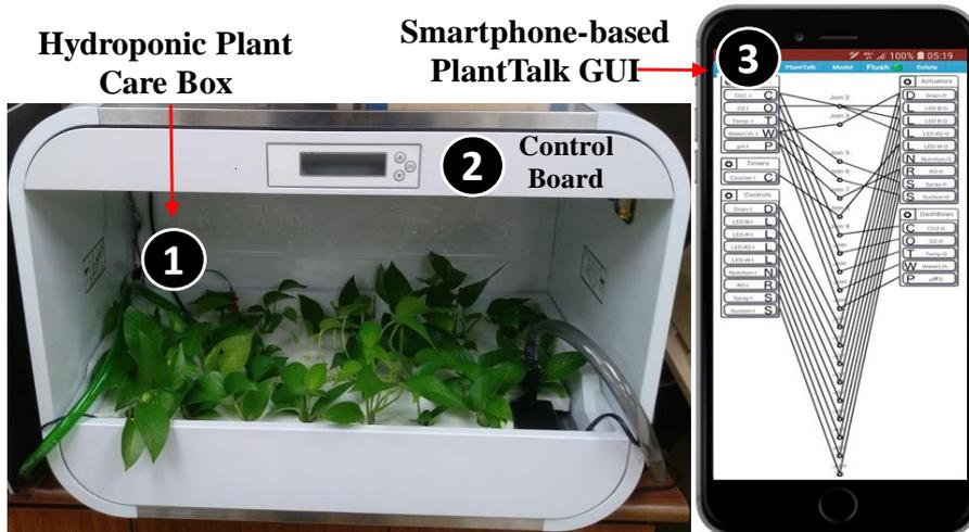
Figure 1. The hydroponic plant box and the PlantTalk GUI.
