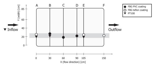
**Figure 2.** The position of the FBG fibers and PT100 sensors on the PVC frame: The top view. The data from the highlighted section are displayed in the results.
