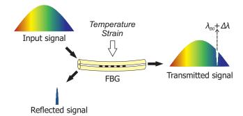
Figure 1. The basic sensing principle of an fiber Bragg grating (FBG) sensor.
