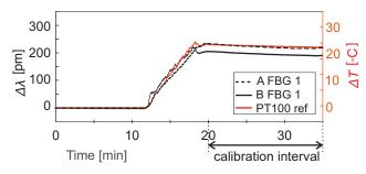
**Figure 5.** An example of the calibration curves for two FBG sensors: Each sensor is inscribed in a fiber with a different coating. The sensor A FBG 1 has a teflon coating; the sensor B FBG 1 has a PVC coating.
