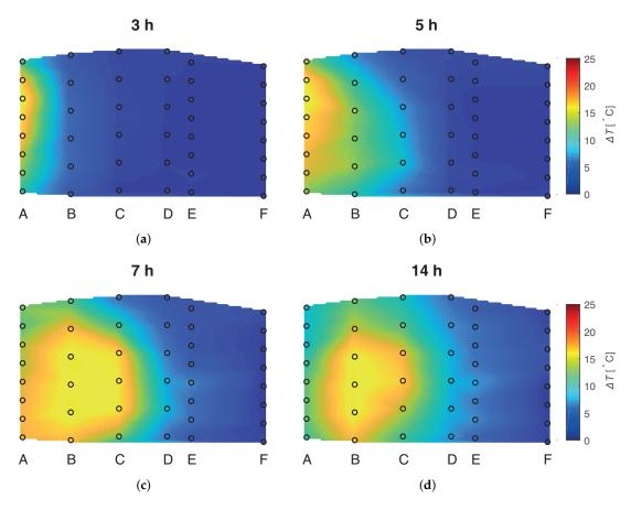
**Figure 7.** The time evolution of the thermal plume in the AS at four different moments: (**a**) t = 3 h; (**b**) t = 5 h; (**c**) t = 7 h; (**d**) t = 14 h from the start of the experiment. The black circles indicate the calculated temperature from the FBG sensors. The displayed temperature map was generated by a linear interpolation from the FBG data.
