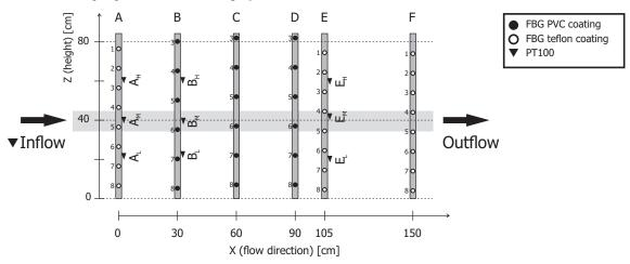
Figure 3. The position of all FBG and PT100 sensors in the aquifer simulator (AS): The side view.
