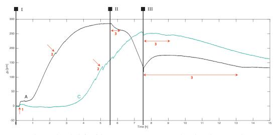
**Figure 8.** The wavelength shifts of the FBG sensors in rows A and C: The red arrows indicate strain events resulting from (1) setup adjustments, (2) local flow, or (3) global flow changes. The Roman numerals demarcate the different experimental stages consistent with Figure 6.
