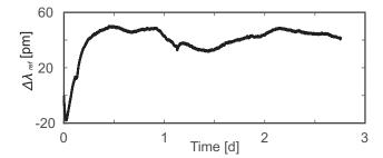
**Figure 4.** The long-term wavelength drift of the FBG interrogator at 1550 nm as measured with a temperature-controlled FBG sensor.
