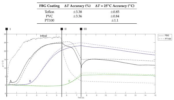
**Figure 6.** A comparison of the FBG data translated into temperatures with the PT100 temperature profiles: The displayed data are from the sensors highlighted in Figure 3. Identical colors indicate sensors in the same row on the frame (the same distance from the inflow system). Experimental stages: I—hot inflow, II—cold inflow, and III—no inflow.
