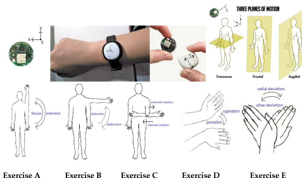
Figure 1. Wristband with BLE-compliant sensor corresponding to local and global coordinates, and the designed simple exercises: A. flexion-extension, B. abduction-adduction, C. external-internal rotation, D. pronation-supination, E. ulnar-radial deviation.
