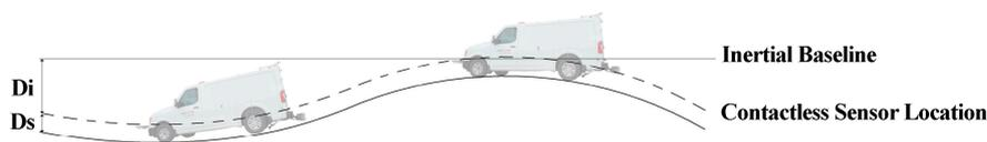
Figure 1. Basis of the inertial profiler.
