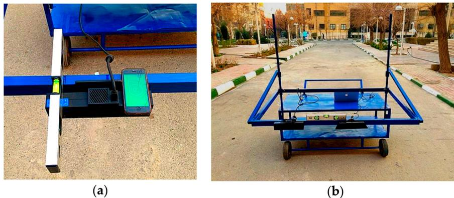
**Figure 3.** (a) Leveling the RGB-D sensor and (b) the data collection cart.
