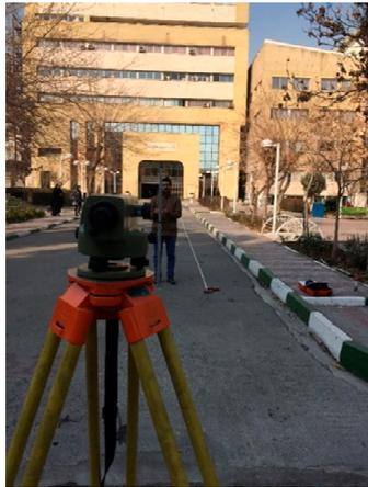
**Figure 7.** Data collection with the rod and level for the validation purpose.
