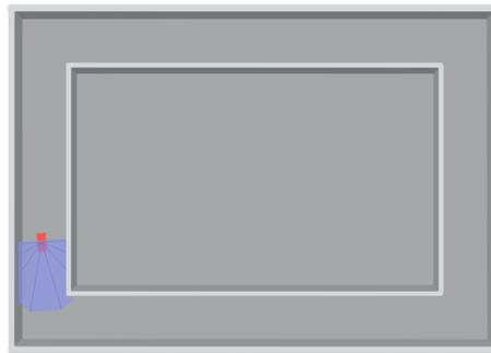
**Figure 6.** Obstacle avoidance task. The agent measures distance from obstacle with 8 sonars. The purpose is trying to go as far as possible without any collision.
