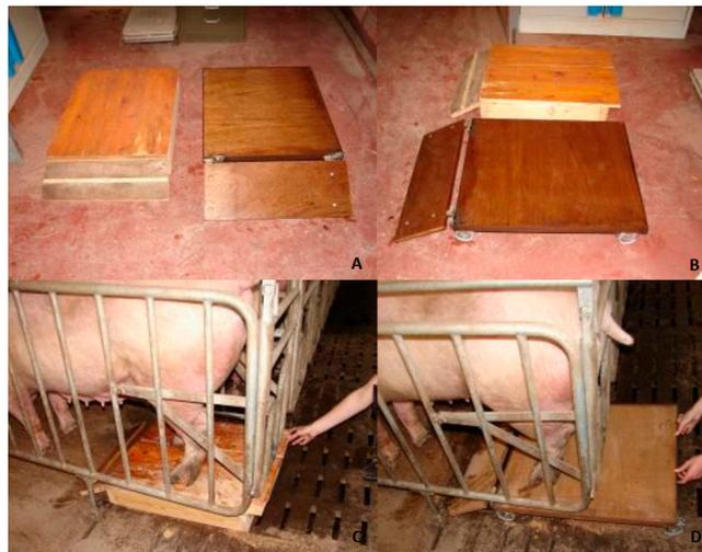
**Figure 2.** First and second wooden prototypes of the Mobile Claw Scoring Device (MCSD). (A,B) = top and side views of the prototypes. The left MCSD is the first and the right MCSD the second prototype. (C) The first wooden prototype tested in a gestation crate. (D) The second wooden prototype tested in a gestation crate.
