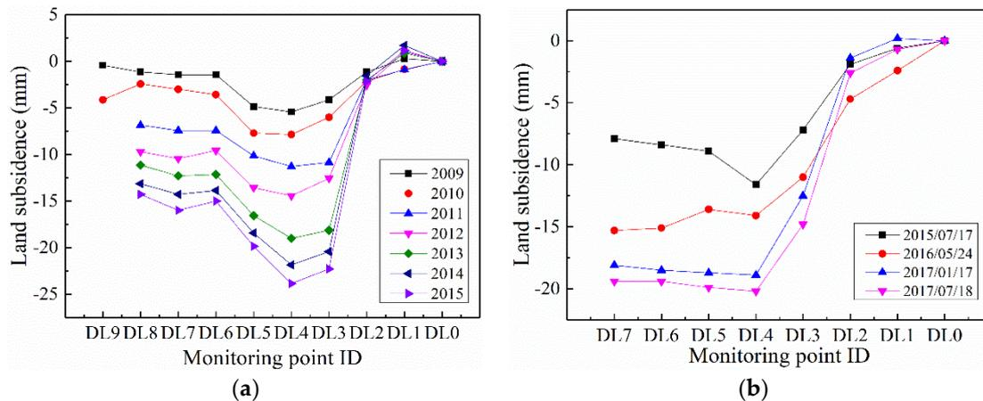
**Figure 10.** The variance of subsidence on the survey line profile with different monitoring times, based on (a) GPS and (b) TLS methods.
