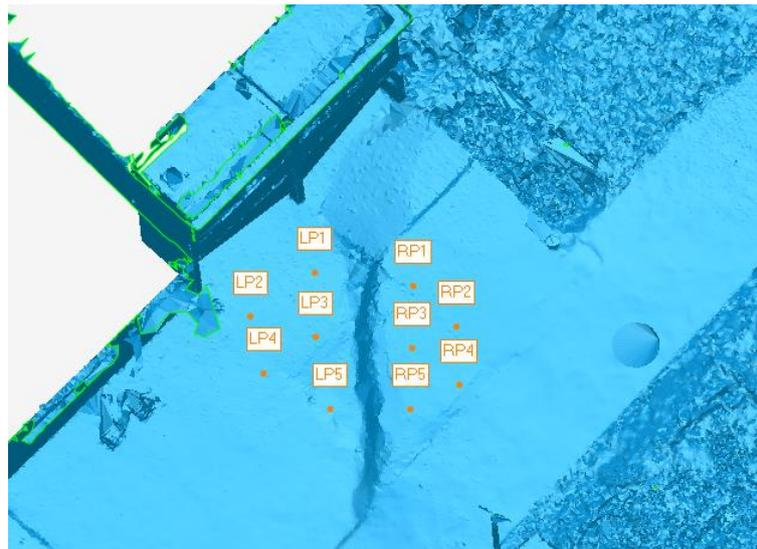
**Figure 6.** The locations of ten monitoring points installed on the left side (denoted as LP) and right side (denoted as RP) of the scarp.
