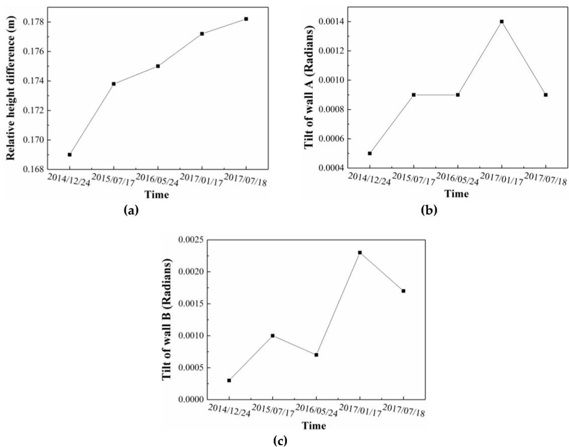
**Figure 7.** The variance of (a) relative height difference, (b) tilt of WA, and (c) tilt of WB with the monitoring time.
