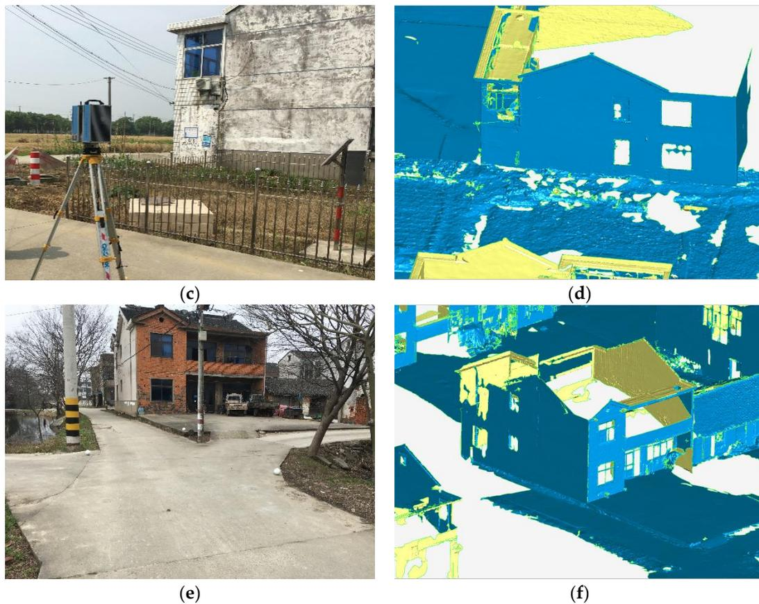
**Figure 5.** The comparison of monitoring objects in site photos and reconstructed modeling: (a,b) scarp, (c,d) wall A, and (e,f) wall B.
