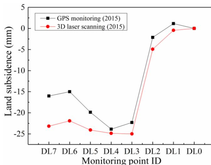
**Figure 11.** Comparison of land subsidence on the survey line in 2015, between GPS and TLS monitoring.
