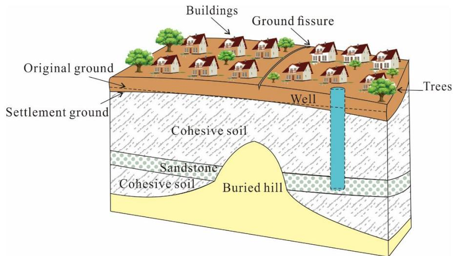
Figure 2. The main formation mechanics of the earth fissure in Wuxi.
