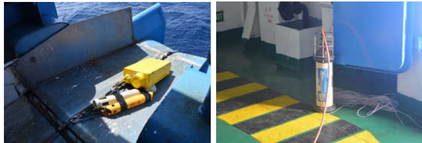
Figure 10. Installation and placement of the transponders (left) and transceiver (right). The transceiver consists of a rugged waterproof electronics bottle connected to a remote acoustic transducer, which was deployed. Lightweight acoustic transponder (Type 8044), operating frequency HF (35–50 kHz), dimensions (length × diameter) 490 mm (19.3") × 63 mm (2.48").
