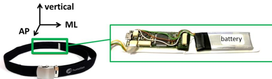
**Figure 2.** Orientation of the sensor system, which is integrated into a belt. The abbreviations stand for mediolateral (ML) and anterior-posterior (AP).
