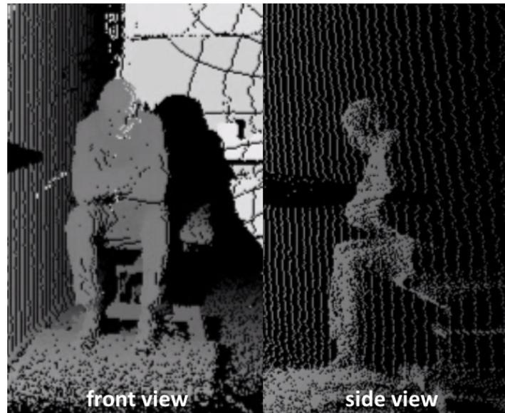
Figure 4. Kinect depth images of the chair rise test in front and side views.
