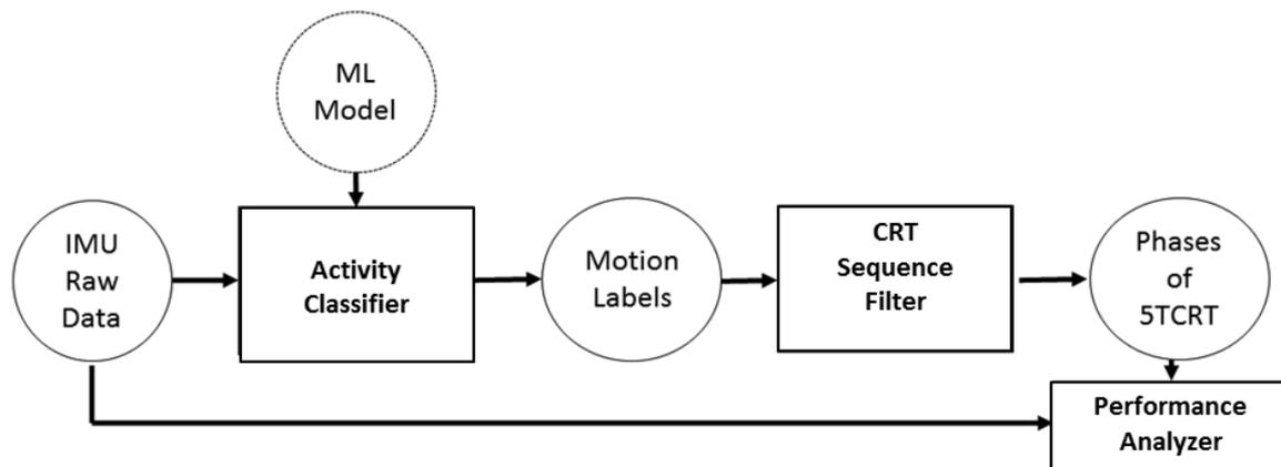
**Figure 6.** Classification- and 5CRT detection-workflow. The system combines a machine-learning based activity classifier, a rule-based model for test detection and algorithms for performance analyses.
