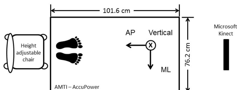
**Figure 3.** Orientation and dimension of the AMTI AccuPower force plate. The chair for the five time chair rise test is placed beside the plate. The abbreviations stand for mediolateral (ML) and anterior-posterior (AP). A Kinect camera is used as optical reference system.
