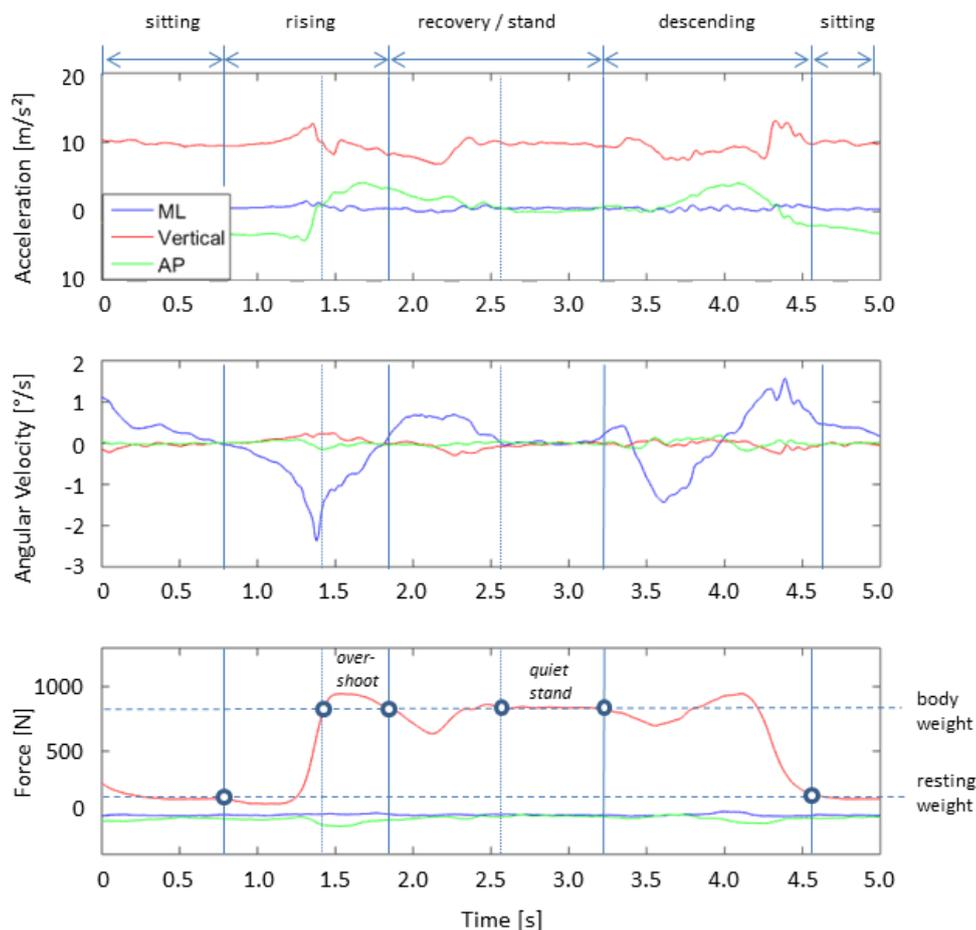
**Figure 11.** Pattern of a typical chair rise test cycle. The figure above shows the accelerometer data in the three directions over time. The figure below shows the force over time during the same sequence. The single phases are marked above.
