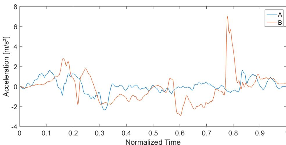
**Figure 19.** Comparison of IMU accelerometer data of participants A and B for the first cycle of the 5CRT.
