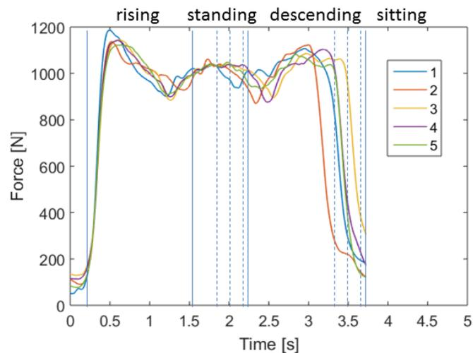
**Figure 13.** Comparison of the 5CRT cycles of one participant based on the force in vertical direction measured by the force plate.
