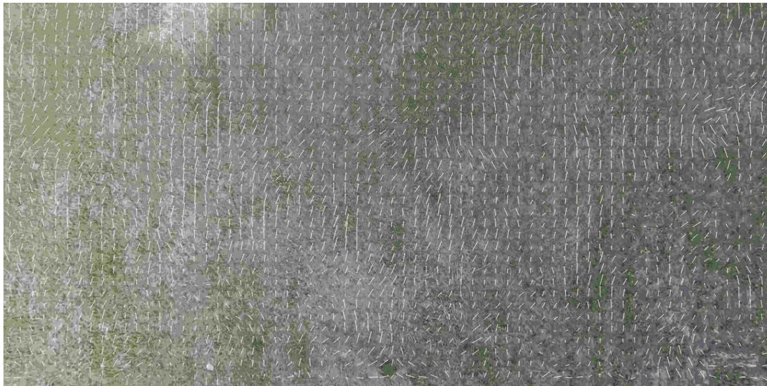
Figure 8. Optical flow estimated by Lucas-Kanade algorithm at the end of glissade, height \approx 30 m, level of averaging 16 \times 16 . By comparing with Figure 6 one can observe much more regular behaviour of the optical flow which gives a better estimation of the flight parameters.
