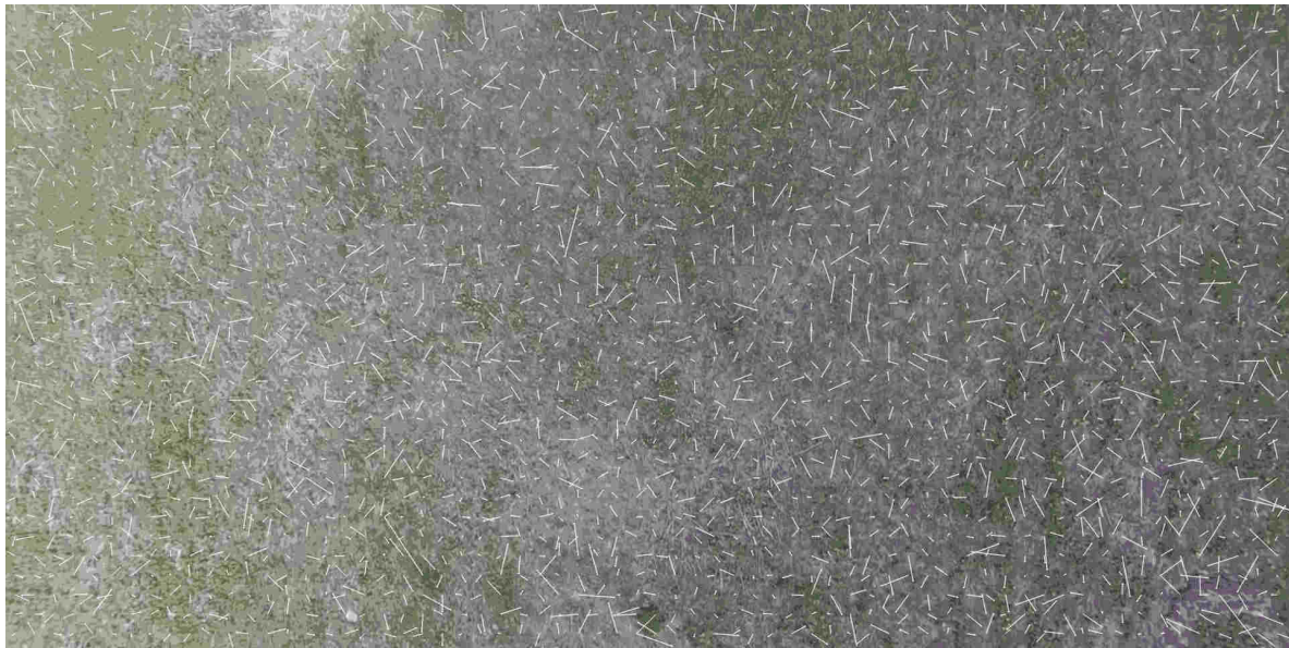
Figure 6. Optical flow estimated by Lucas-Kanade algorithm at the end of glissade, height \approx 30 m, level of averaging 2 \times 2 . One can observe the very chaotic nature of the optical flow which prevents the estimation of the flight parameters.
