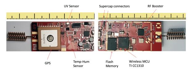
Figure 2. Sensor board components placement.
