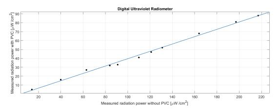
**Figure 6.** Relationship between the intensity of UVB detected by the digital ultraviolet radiometer outside and inside the PVC case. Each point corresponds to a different time of the day. Linear fit is also plotted.
