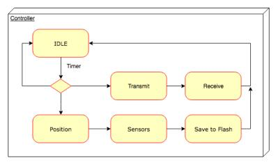
Figure 12. Simplified Finite State Machine of the controller.
