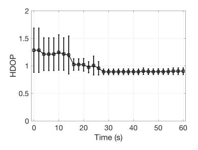
**Figure 14.** Distribution of the Horizontal Dilution of Precision (HDOP) as a function of the time from the first fix.
