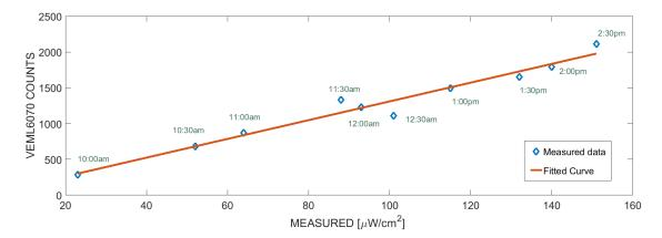
**Figure 7.** Calibration curve of VEML6070 sensors at different daytime, the measured intensity of UVB has been obtained by an ultraviolet radiometer. Linear fit is also shown.
