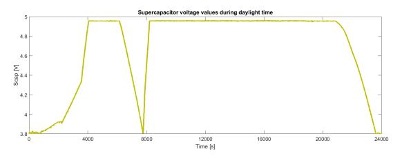
Figure 11. Behavior of the voltage of the supercapacitor during continuous operation.
