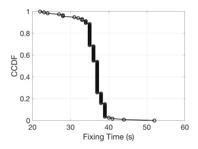
**Figure 13.** Complementary cumulative distribution function of the time to obtain the first fix from the GPS unit.
