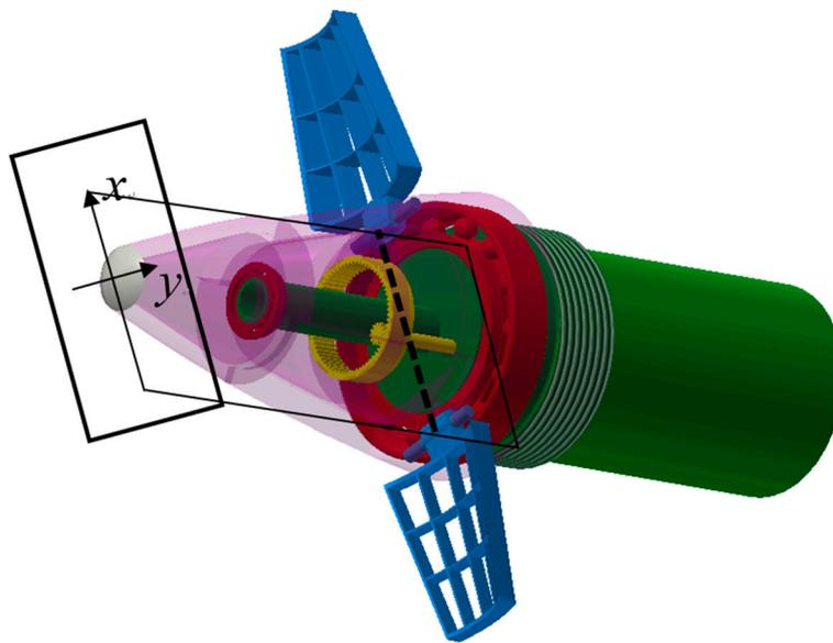
**Figure 2.** Maneuvering components in forward fuze.
