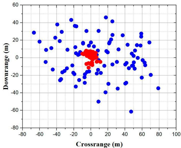
Figure 14. Deviation between impact points and target for ballistic and corrected trajectories.
