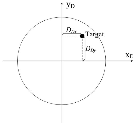
**Figure 9.** Schematic of the deviation in the detector coordinate system.
