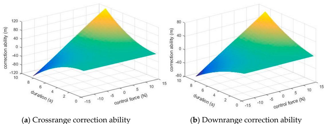
Figure 7. The correction ability with control force and duration.
