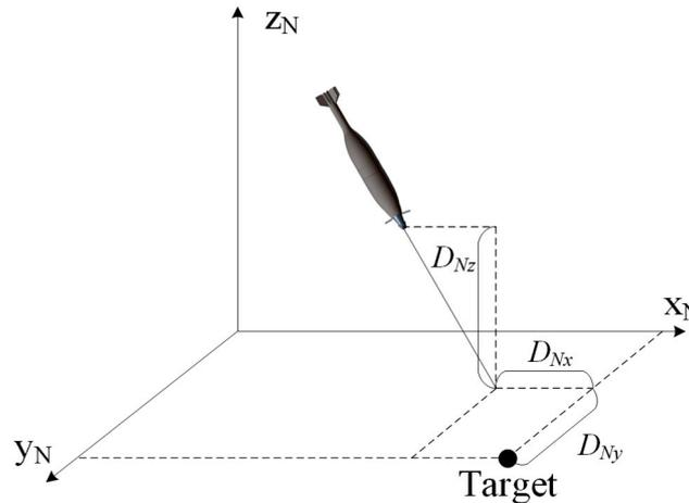
Figure 8. Schematic of the deviation in the inertial coordinate system.
