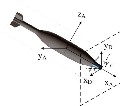
Figure 4. The detector coordinate system.
