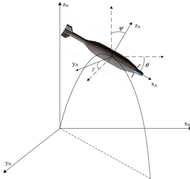
Figure 3. Inertial and body-fixed coordinate systems.
