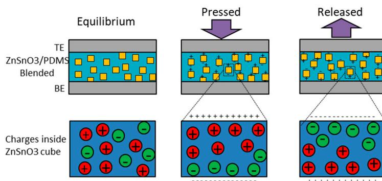
**Figure 5.** Working mechanism of the  $\text{ZnSnO}_3$ :PDMS-based nanogenerator.
