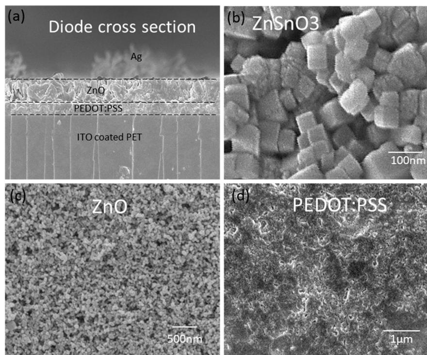
**Figure 4.** (a) Cross sectional view of the ITO/PEDOT:PSS/ZnO/Ag device. (b) Zinc stannate. (c) ZnO thin film SEM image. (d) PEDOT:PSS thin film SEM image.
