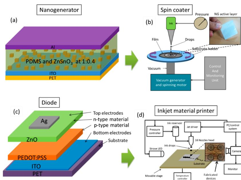
**Figure 2.** (a) NG layout diagram fabricated layer by layer. (b) NG fabrication with a spin coater. (c) Materials layout diagram of the diode device. (d) Schematic diagram of the inkjet material printer.
