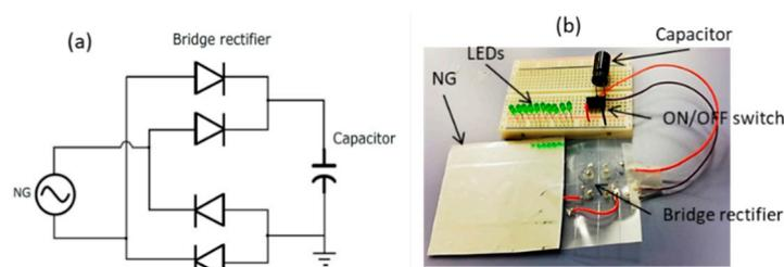
**Figure 3.** (a) Schematic diagram of the NG connected with bridge and storage capacitor. (b) Digital photograph of the fabricated system.
