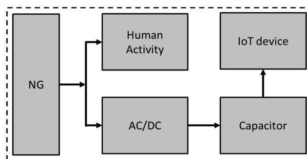
Figure 1. Block diagram of the people counting and motion sensor.
