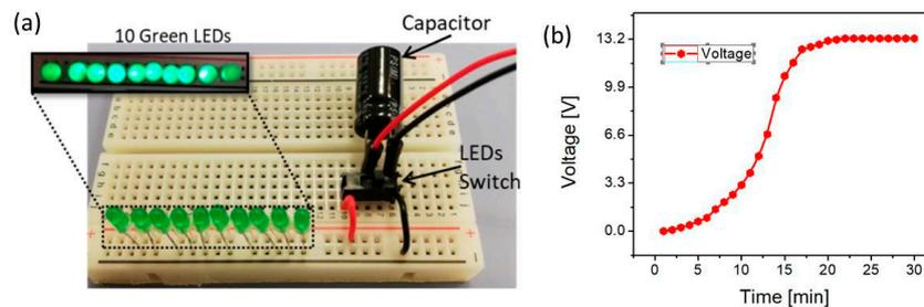
**Figure 7.** (a) 10 green LEDs glowed with harvested energy. (b) Harvested voltage across the capacitor.
