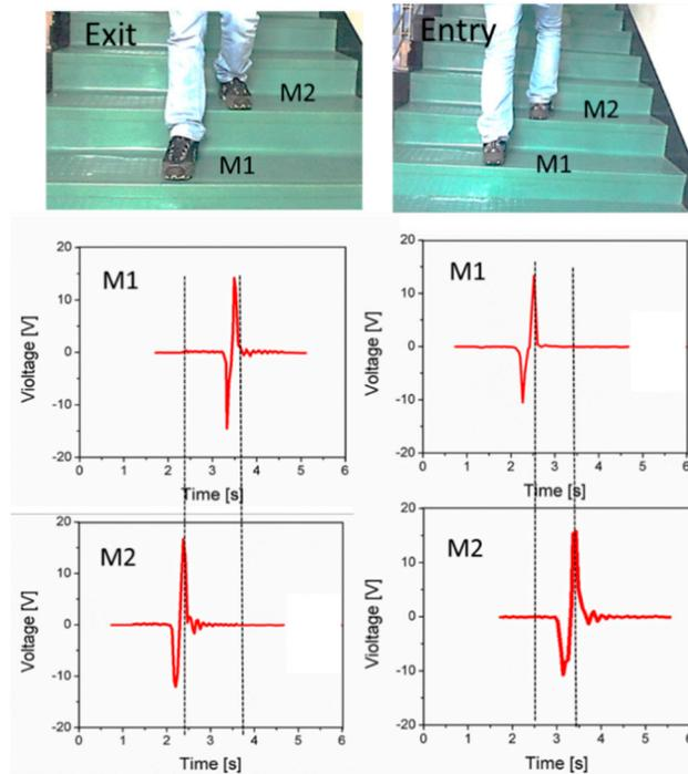
**Figure 8.** People counting application of the proposed device, in the Exit scenario: M2 is pressed prior to M1 the voltage spikes occurs at 2.5s for M2 and 3.5s for M1 in the time domain. In the Entry scenario: M1 generates voltage spike at 2.5s while M2 at 3.5s.
