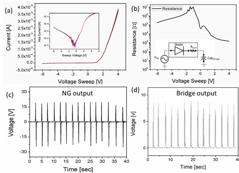
**Figure 6.** (a) I-V curve of the diode. The inset shows the absolute current graph of the diode. (b) Diode resistance against the sweep voltage. (c) NG output voltage against human footsteps applied for 40 s. (d) Output voltage at the bridge rectifier.
