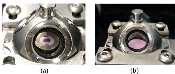
**Figure 1.** Pictures of the Cu-PAN samples in the gas measurement chamber dome: (a) Colored silica powder before gas exposure. (b) Cu-PAN layer printed on coated paper before gas exposure.
