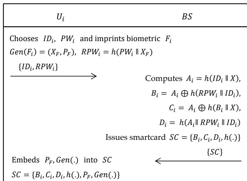
Figure 2. Registration phase of Ali et al.'s scheme.
