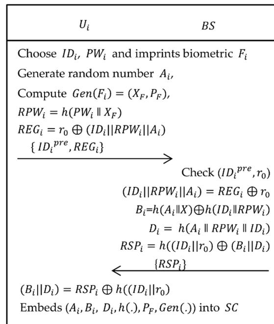
Figure 5. User registration phase of the proposed scheme.
