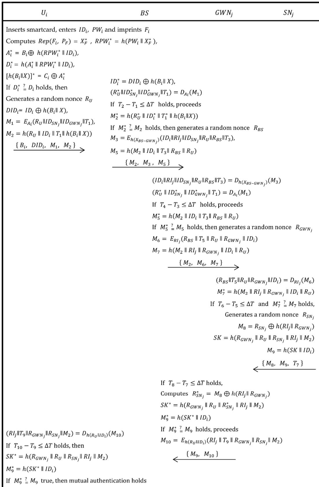
Figure 3. Login, authentication and key agreement phase of Ali et al.’s scheme.
