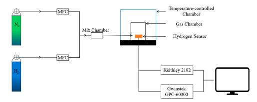
Figure 4. Schematic of the hydrogen measuring system.
