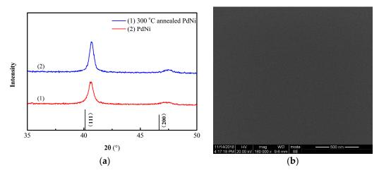
**Figure 5.** (**a**) X-ray diffraction (XRD) patterns of (1) PdNi and (2) 300 °C annealed PdNi film; (**b**) SEM image of PdNi thin film.
