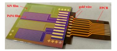
Figure 3. Photo of the fabricated hydrogen sensor.
