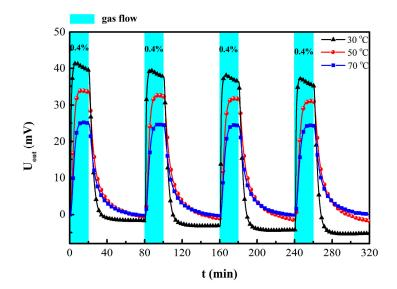
Figure 6. Repeatability of the hydrogen sensor at 30 °C, 50 °C and 70 °C under 0.4% H<sub>2</sub>.
