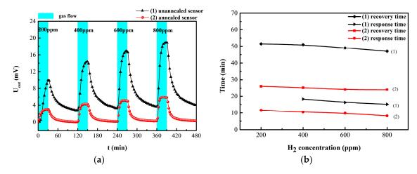
**Figure 7.** (a) Response curve of (1) unannealed sensor and (2) annealed hydrogen sensor at 50  $^{\circ}$ C under different H<sub>2</sub> concentrations; (b) the response time and recovery time of (1) and (2).
