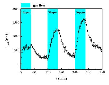
Figure 8. Response curve of the annealed hydrogen sensor at 50 °C.
