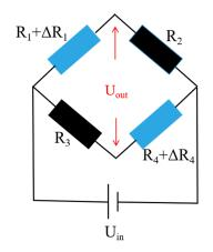
Figure 2. Structure diagram of Wheatstone bridge type hydrogen sensor.
