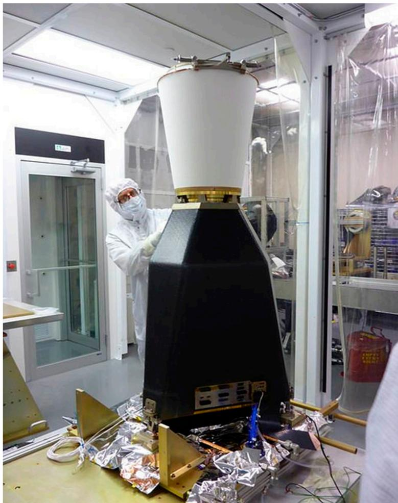
Figure 1. GLM assembly with sun shade pre-launch [23].
