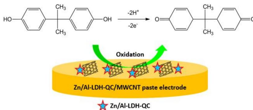
**Scheme 1.** The electro-oxidation reaction of bisphenol A on electrode surface during electrochemical sensing.
