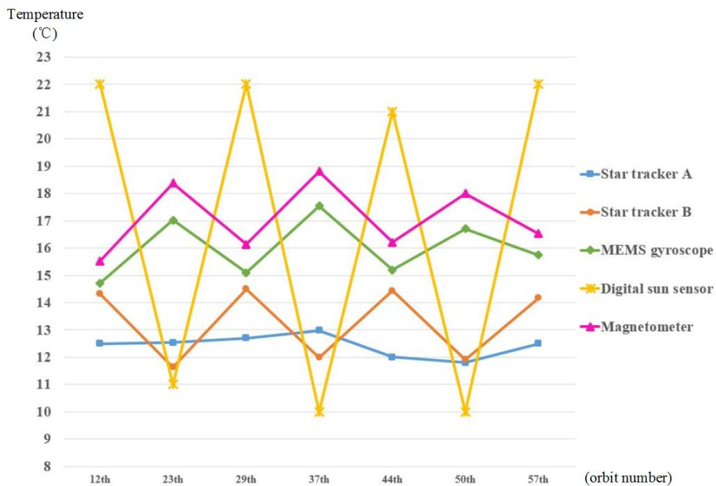
Figure 16. Temperature variation curve of the outside instruments in the Luojia 1-01.
