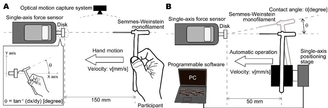
**Figure 1.** Experimental measurement apparatus: (A) under manual (human) operation, hand motion during monofilament application is measured using an optical 3D motion capture system, and the monofilament buckling force is measured using a single-axis force sensor; (B) under automated operation, the monofilament is applied using a single-axis positioning stage controlled by a stepping motor and a personal computer with programmable software.
