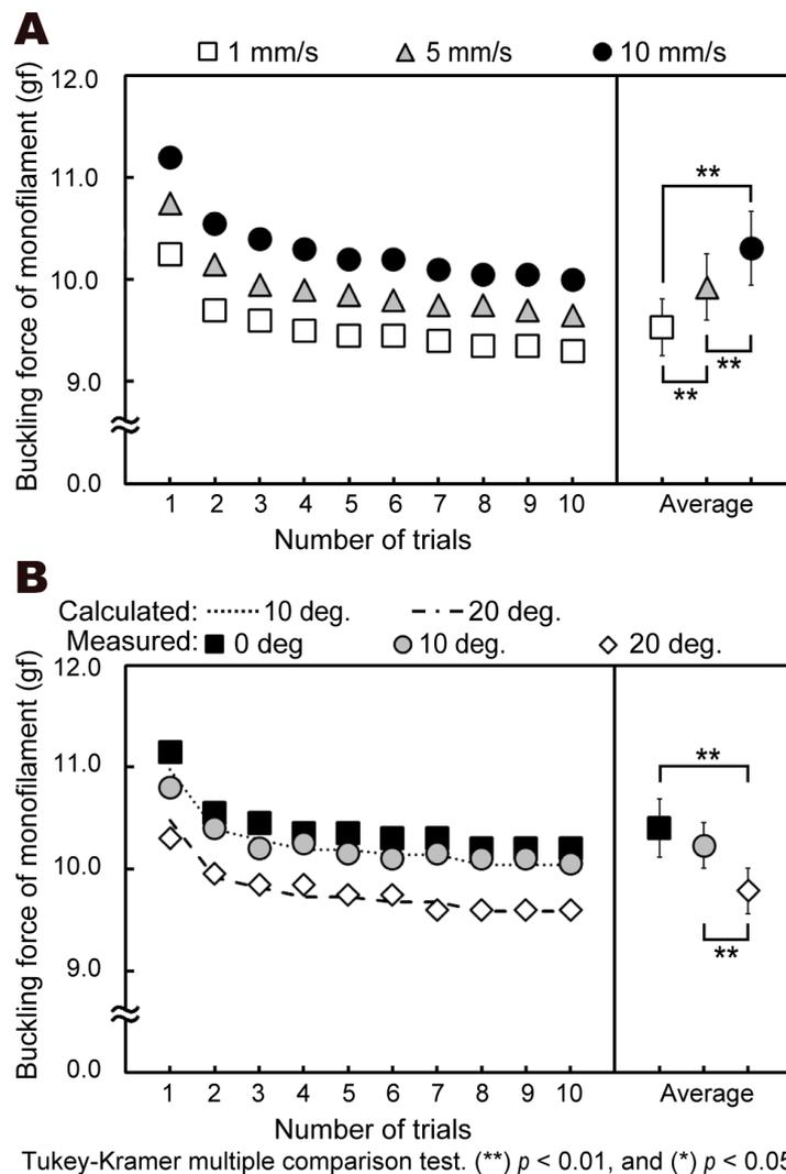
**Figure 4.** Experimental buckling force results for different operational scenarios under automated operation using the multi-use monofilament: (A) positioning stage velocities of 1, 5, and 10 mm/s; (B) monofilament contact angles of 0°, 10°, and 20°.
