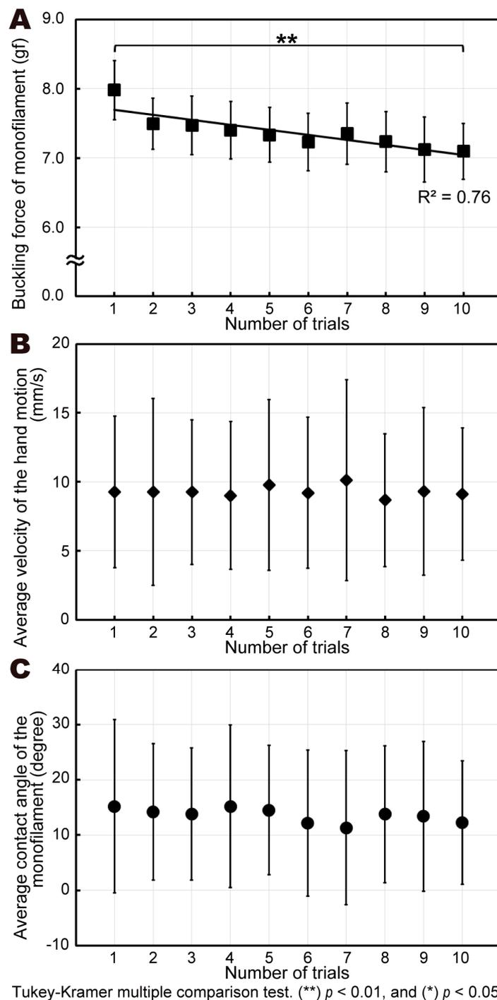
**Figure 3.** Experimental results of manual (human) operation: (A) monofilament buckling forces for each trial; (B) average velocity of human hand motion; (C) average contact angle of the monofilament.
