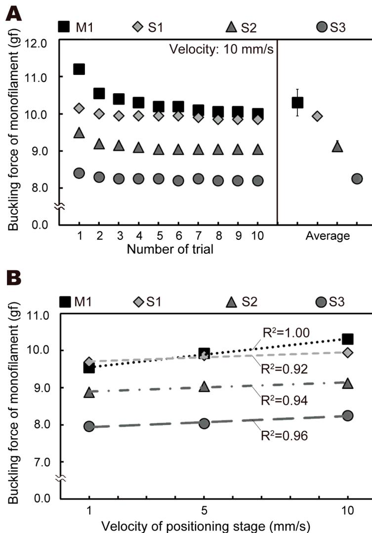
**Figure 5.** Experimental buckling force results for different monofilament types under automated operation using all four monofilaments, with one multi-use monofilament (denoted M1) and three single-use monofilaments (denoted S1, S2, and S3): (A) for each trial and (B) as a function of positioning stage velocity.
