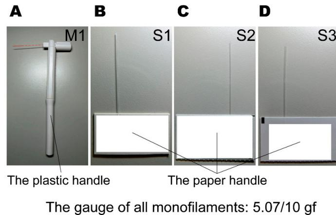
**Figure 2.** The total four 5.07/10 gf monofilaments: (A) the multi-use monofilament (M1); (B–D) the single-use monofilaments (S1, S2, and S3).
