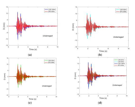
**Figure 9.** The displacement time-history responses as collected by SPs compared with LDSs using different sampling rates of (**a**) 100 Hz, (**b**) 50 Hz, and (**c**) 25 Hz. (**d**) A comparison of all sampling rates.
