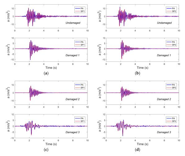
**Figure 4.** The acceleration time-history responses, as collected by the piezoelectric accelerometers (PAs) and smartphones (SPs) for four damage cases subjected to Nr-1 cm excitation, are compared. Representative results from (**a**) frame 1 and (**b**) frame 2 in the undamaged and damaged 1 cases, as well as (**c**) frame 1 and (**d**) frame 2 in the damaged 2 and damaged 3 cases are overlaid.
