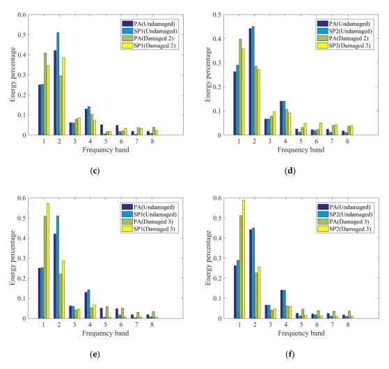
**Figure 10.**  $p_j$  calculated for (**a**) frame 1 and (**b**) frame 2 in the damaged 1 case, (**c**) frame 1 and (**d**) frame 2 in the damaged 2 case, and (**e**) frame 1 and (**f**) frame 2 in the damaged 3 case when structure is subjected to Nr-1 cm excitation.
