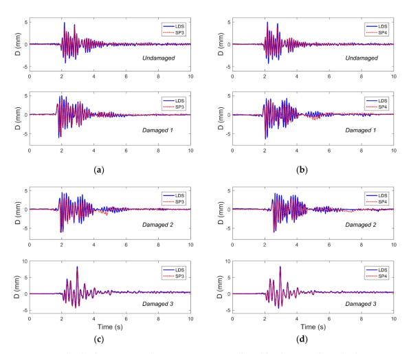
**Figure 7.** The displacement time-history responses as collected by the LDSs (laser displacement sensors) and SPs with Nr-1 cm excitation for four damage cases are compared and found to show good agreement. Representative results are shown from (**a**) frame 1 and (**b**) frame 2 in the undamaged case and damaged 1 case, as well as from (**c**) frame 1 and (**d**) frame 2 in the damaged 2 and 3 cases.
