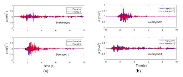
**Figure 6.** The Y-axis acceleration time-history responses as collected by smartphones subjected to Nr-1 cm are shown (**a**) in the undamaged and damaged 1 cases and (**b**) in the damaged 2 and 3 cases.
