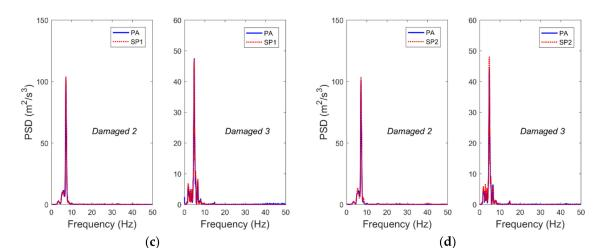
**Figure 5.** Using the acceleration time-history measurements from Figure 4, the power spectral density functions of (**a**) frame 1 and (**b**) frame 2 in the undamaged and damaged 1 cases, as well as (**c**) frame 1 and (**d**) frame 2 in the damaged 2 and damaged 3 cases are compared.
